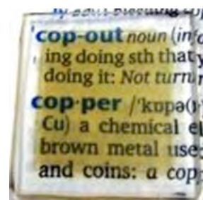
Fig. 1 Photograph of p -type \text{Cu}_2\text{O} thin film fabricated by molecular precursor method
